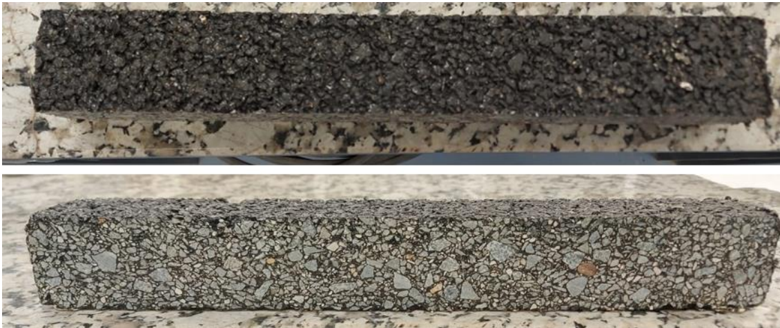
Figure 24. Surface and internal appearance of SMA 8
