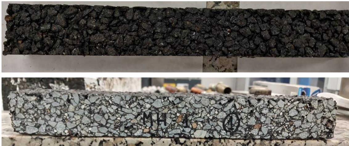
Figure 22. Surface and internal appearance of OSMA 11
