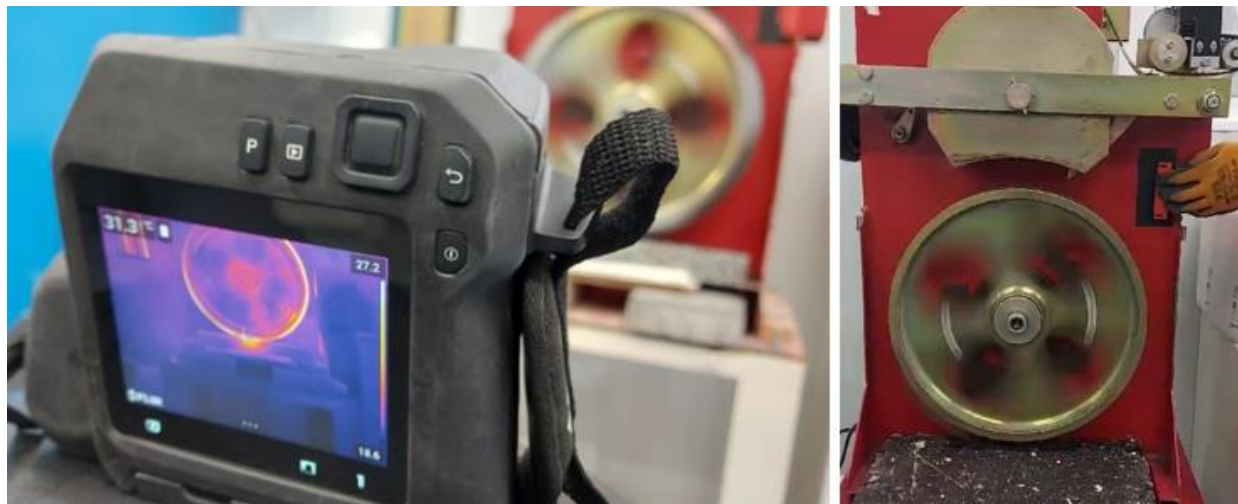
Figure 16. Accelerated Polishing Machine adaptation to analyse the asphalt-tyre interaction
