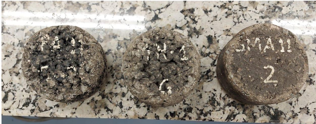
Figure 28. Example of the appearance of the asphalt samples after the Cantabro test
