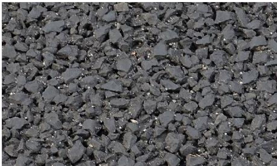
Figure 12. Surface view of special Hybrid Mix pavement in Matsui in Japan. It looks like a PA but it is actually not permeable
