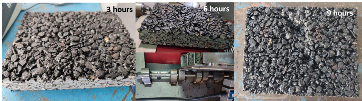
Figure 25. Visual appearance of PA 11 mixture, left) after 3 hours of testing testing, middle) after 6 hours of testing and, right) after 9 hours of testing
