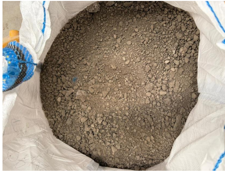
Figure 15. Steel slag appearance
