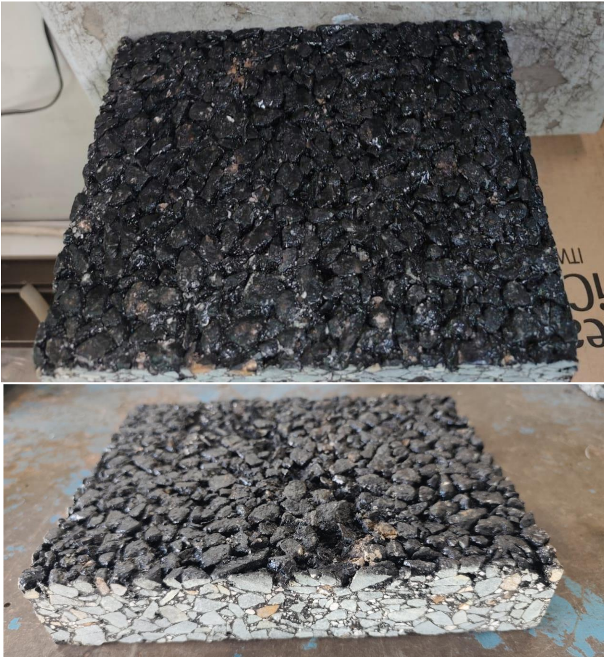
Figure 26. Visual appearance of OSMA 11 mixture. Top) Before testing, Bottom) after testing
