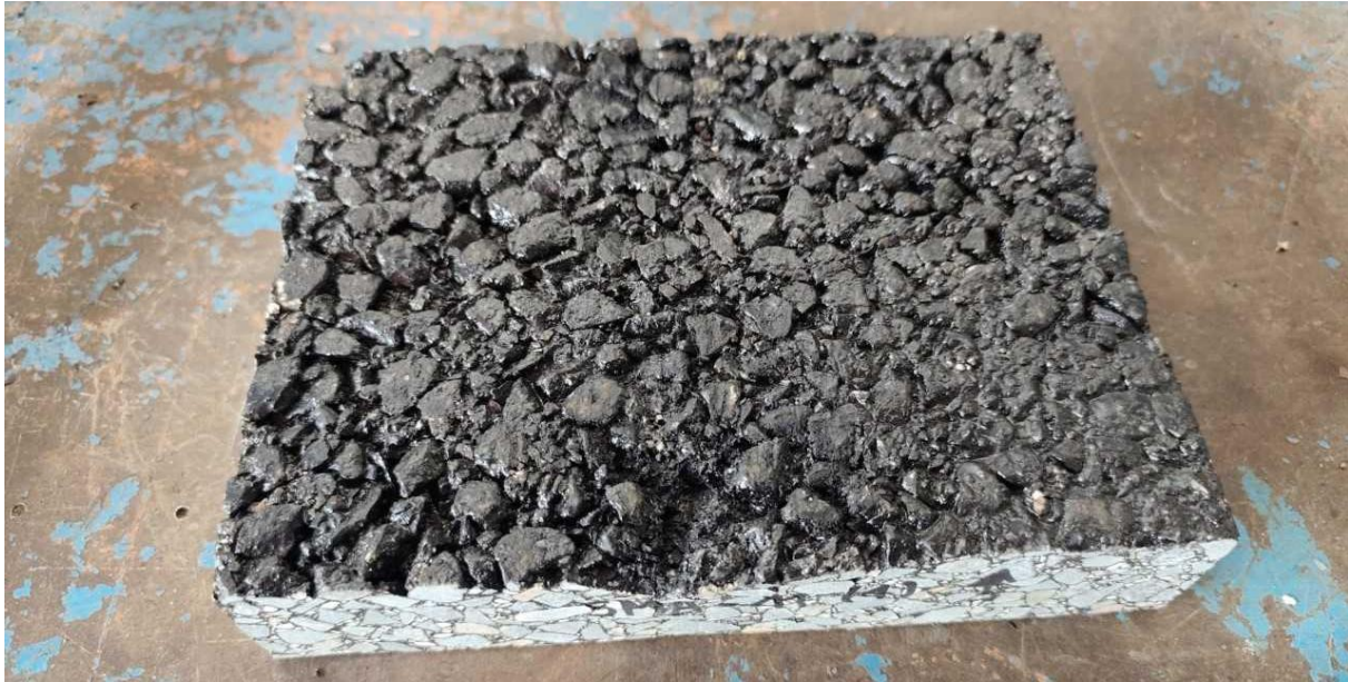
Figure 27. Visual appearance of SMA 11 mixture (Top) before testing, (bottom) after testing
