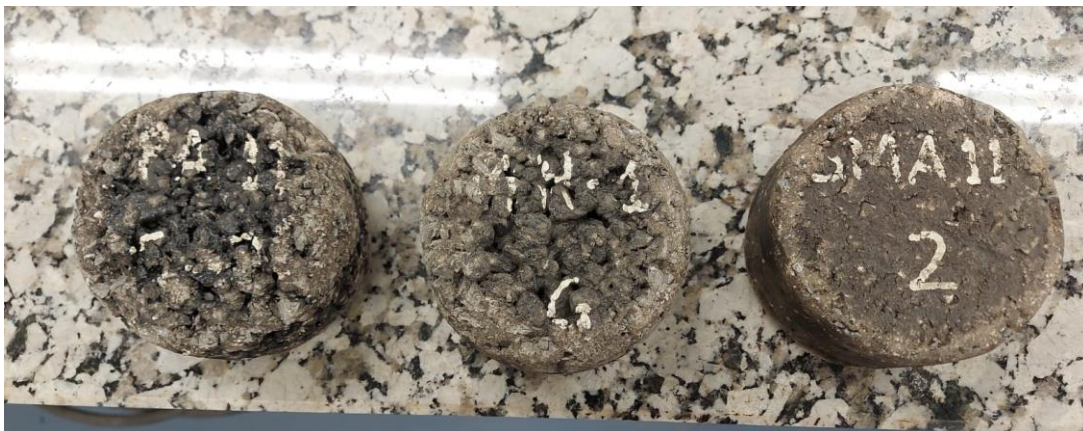
Figure 4. Appearance of asphalt samples after Cantabro test (extracted from D2.4)
