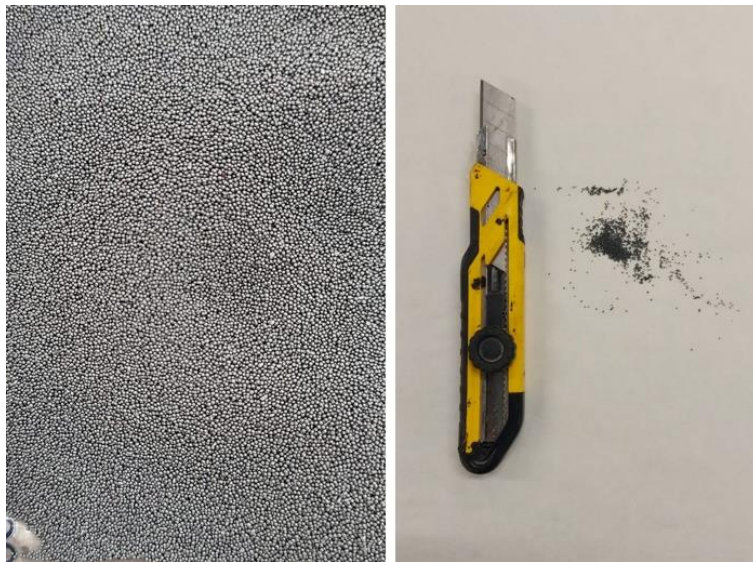
Figure 16. Steel spheres additives – Appearance and relative dimensions
