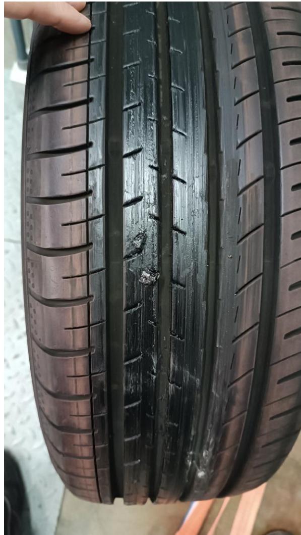
Figure 17 Tire surface degradation after 9 hours of tests
