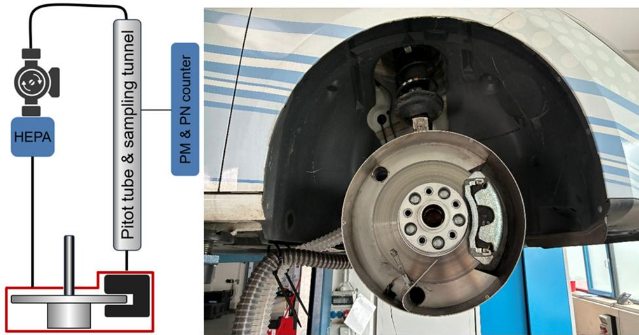
Figure 3 left: Scheme of the setup utilized for brake emission measurements on the brake and on the chassis dynamometer. Right: Housing mounted on front wheel.
