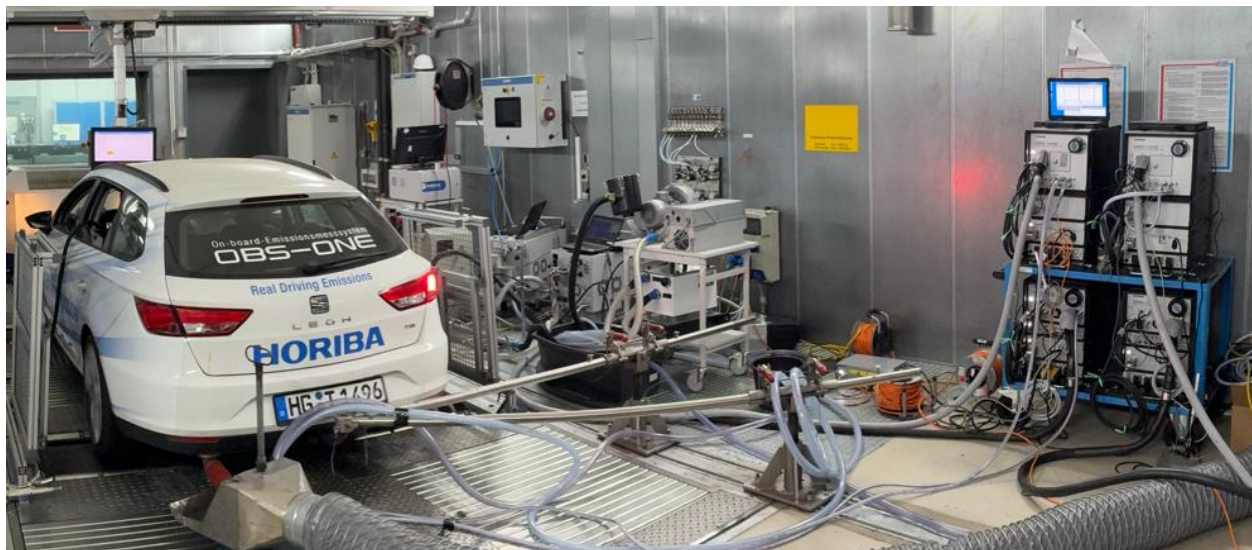
Figure 4 Vehicle with brake enclosure on chassis dynamometer. On the right side of the image pump, filters and all 9 measurement equipment units can be seen
