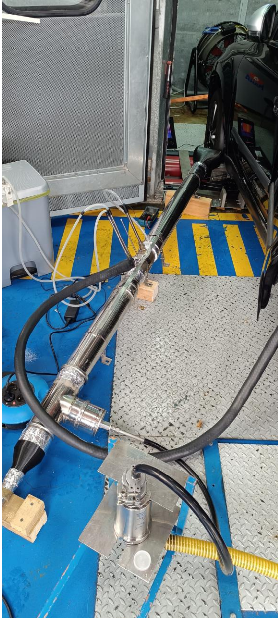
Figure 8 Experimental setup for tire-road emission measurements.
