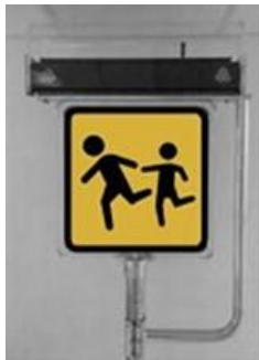
Figure 19 The intelligent bus stop (IBS) activated by the children's VRU-unit.
